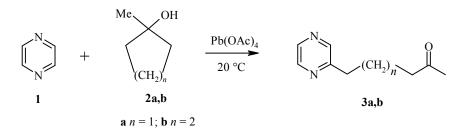
In the present work, a new approach is described for the synthesis of 2-(oxoalkyl)pyrazines (Table 1) based on the reaction of pyrazine 1, 1-methylcycloalkanols 2a,b, and Pb(OAc)<sub>2</sub> upon mechanical activation in a heterogeneous system with the absence of solvent.
